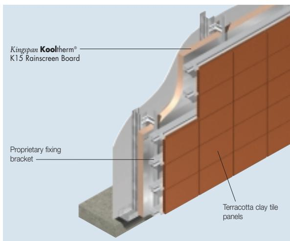
Figure 3 Insulated rainscreen cladding systems on steel frame
