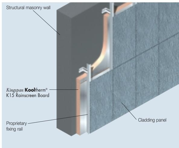
Figure 1 Insulated rainscreen cladding systems (non-proprietary external finish)
